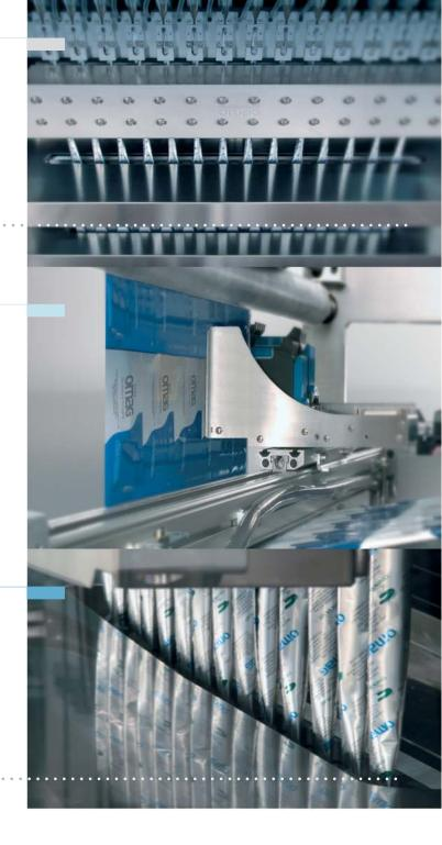
Pick-up Heads by vacuum cups and Stick transfer system to the buckets of a cartoner.
