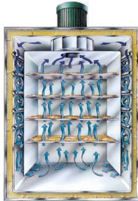
Rapid cooling and drying is achieved by powerful centrifugal fans and internal water cooled heat exchangers.
