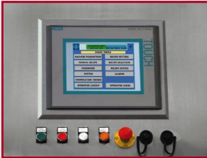
Pannello operatore touch screen Touch screen control panel
