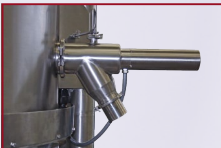
Carico in depressione Vacuum loading
