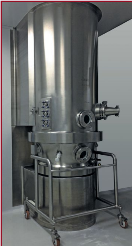
Letto fluido "through wall" Through wall Fluid Bed Dryer
