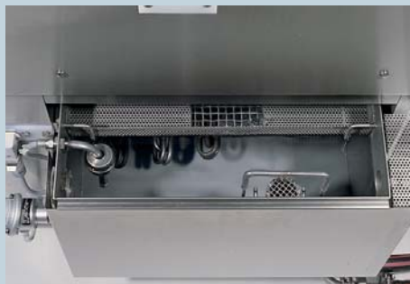
Recirculating pump station
