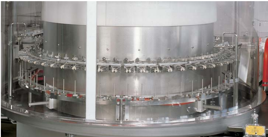
Transfer from the transport grippers into the outfeed system
