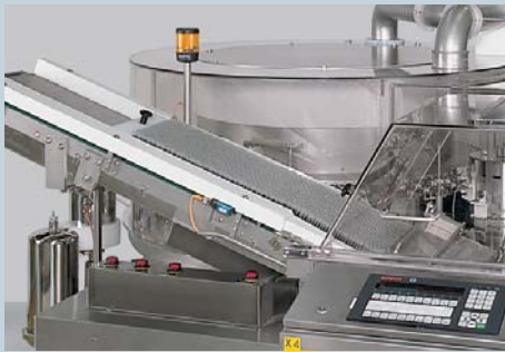
Traying off the containers via a conveyor belt
