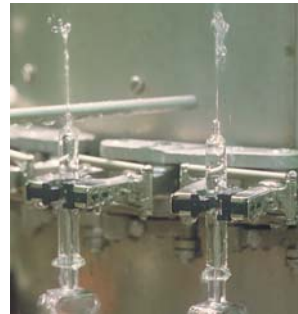
Syringe barrels are thoroughly cleaned inside and outside (jetting needles immerse into the syringe body)
