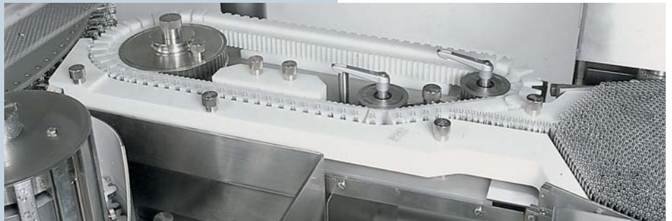
Container discharge via toothed belt as transfer to the sterilizing tunnel
