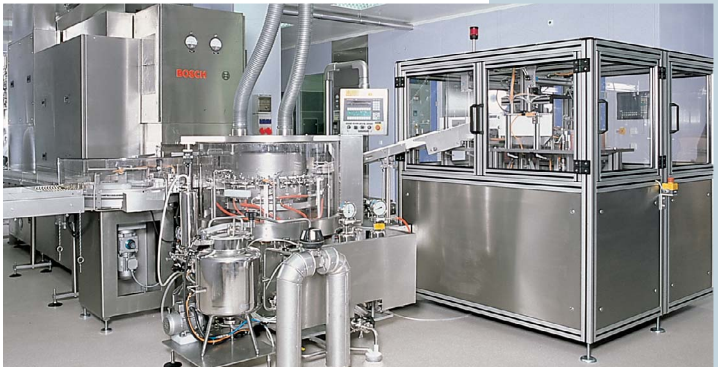
Syringe barrel compact line: Detraying of syringe barrels, cleaning, sterilizing, filling, closing, traying-off
