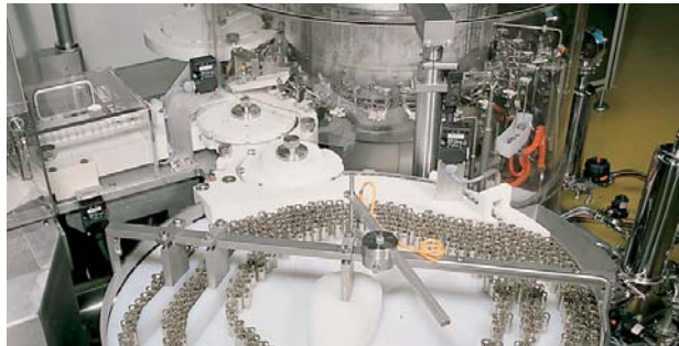
Inserting the syringe barrel into the puck (additional device)
