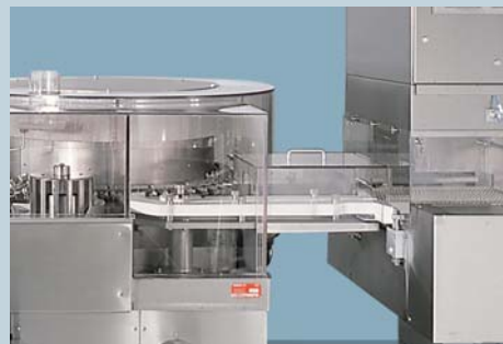
Transfer to one downstream sterilizing tunnel
